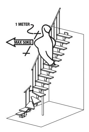
BANISTER LOAD: MAX 50 KG HORIZONTAL LOAD PR 1 METER
